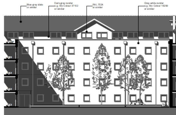
Bldg-Elevation 05 (Courtyard 1)-GA Scale - 1:125
